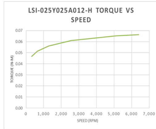
Example of typical use motor speed curve. Higher speeds possible and is dependent on the applied voltage. Top speed may be limited mechanically. Please consult factory if higher speeds are required.
