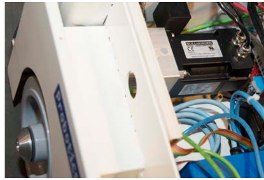
Low voltage motor in an autonomous transportation system. Autonomous transportation systems fitted with low voltage servo axes are characterized by high precision and dynamic driving behavior.
