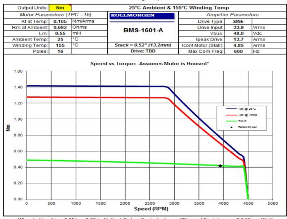
\*Mounted to: 4 in x 3.25 in x 0.25 in AL Heat Sink or Equivalent Rated Speed = 3933 RPM Rated Power (Watts) = 170
