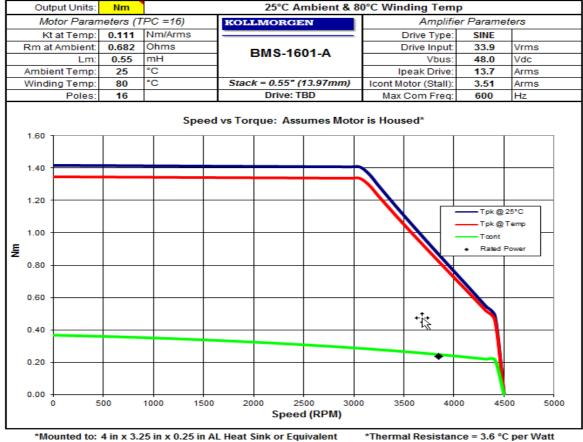
Rated Speed = 3847 RPM Rated Power (Watts) = 95
