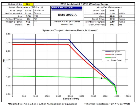
\*Mounted to: 7 in x 7.5 in x 0.75 in AL Heat Sink or Equivale Rated Speed = 3847 RPM Rated Power (Watts) = 374 \*Thermal Resistance = 2.17 °C per Watt Kb (hot)= 7.1 Vrms/kRPM
