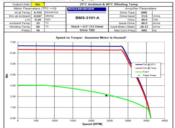
\*Mounted to: 7.5 in x 7 in x 0.375 in AL Heat Sink or Equivalent Rated Speed = 2412 RPM Rated Power (Watts) = 527
