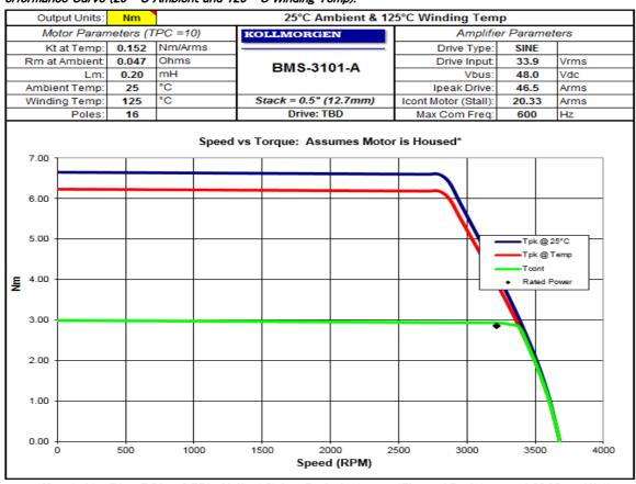
\*Mounted to: 7 in x 7.5 in x 0.75 in AL Heat Sink or Equivalent Rated Speed = 3218 RPM Rated Power (Watts) = 960
