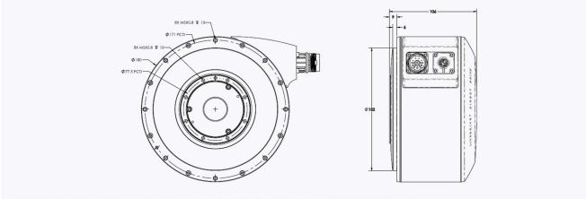
LDD 1830 with M23 and M12 connectors shown. One cable technology (M23 only) on HIPERFACE DSL® models.
