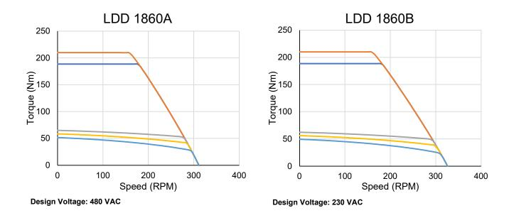
Performance curves assume an ambient temperature of 20°C and heat sink dimensions as stated in Specifications. Temperature rise affects motor performance and is dependent on both the ambient operating temperature and the maximum allowable winding temperature. Contact an Applications Engineer for special thermal or voltage requirements.
