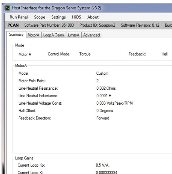
HiDS allows extreme flexibility via simply changing parameters, without the need to reload custom software.
