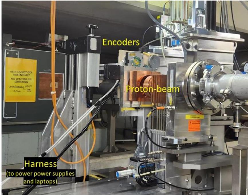
Figure 8 Proton beam SEE irradiation set up
