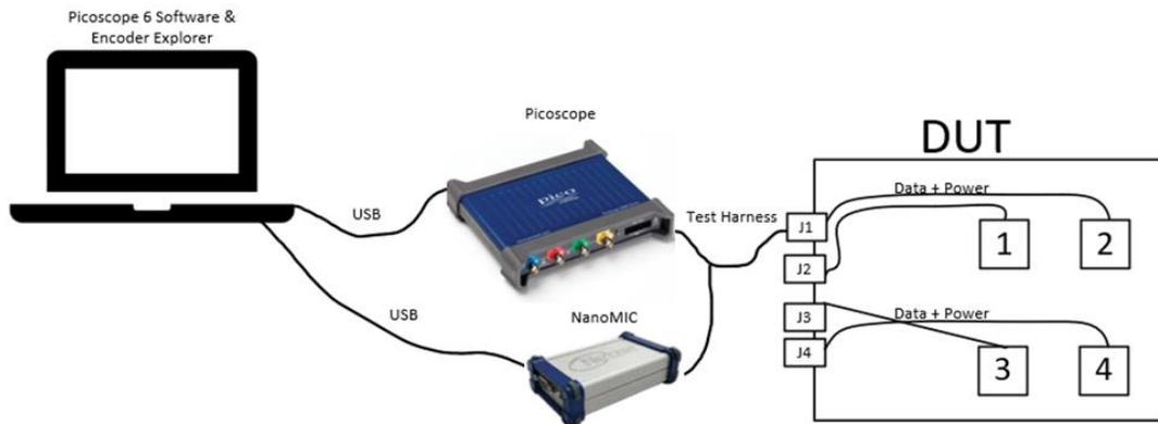
Figure 5 Wiring set up for functional testing
