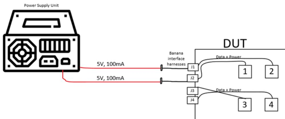
Figure 4 Wiring scheme for DUT irradiation powering
